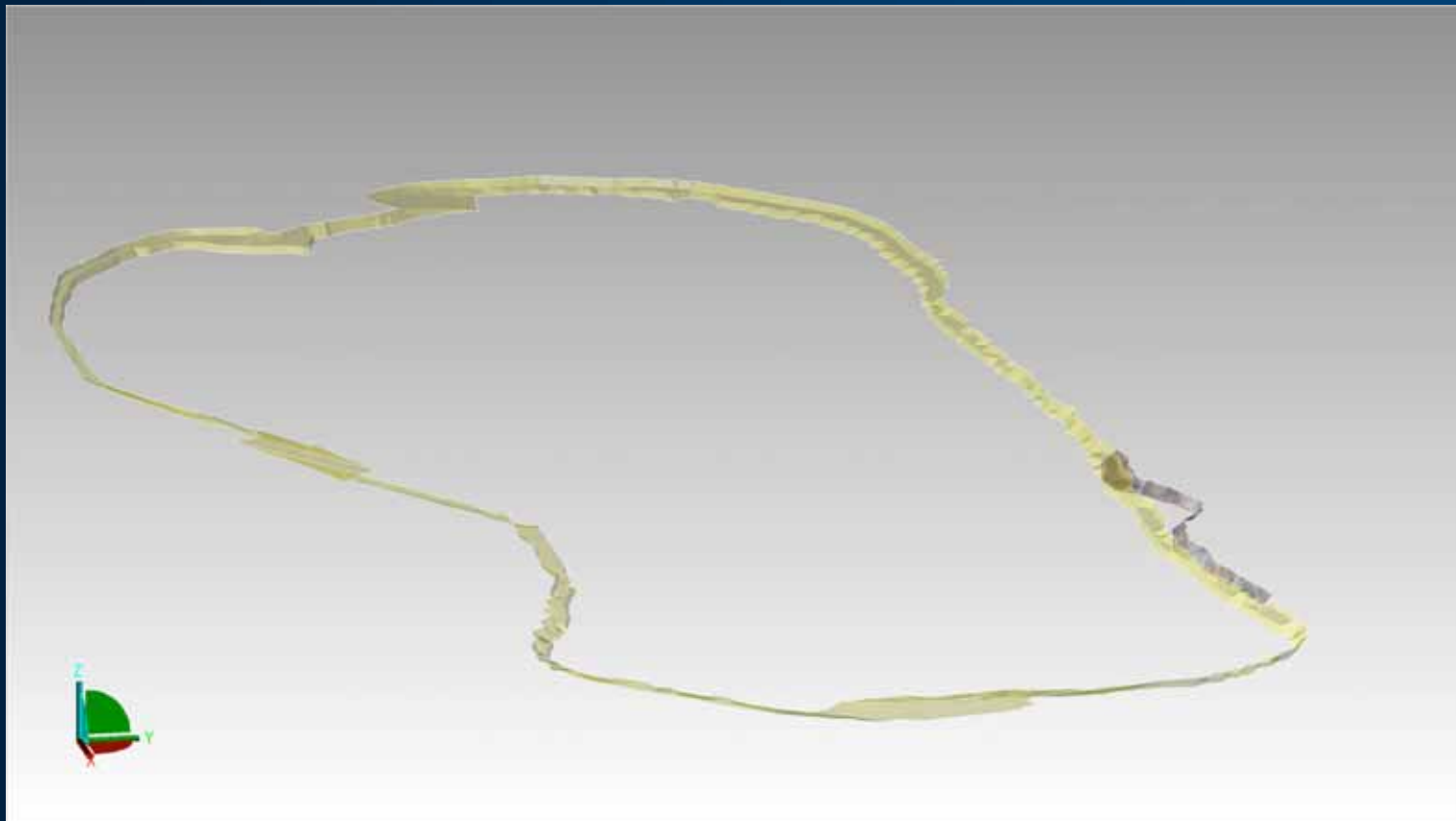
Clipped bench view of the Sirovision surface vs. surveyed pit surface
